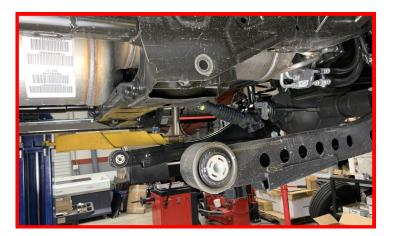
Remove the radius arm lower cam bolt on both sides.
