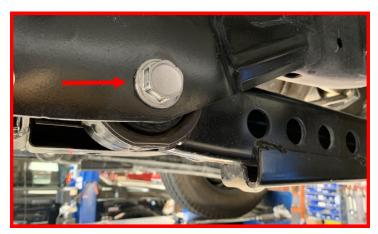
Lower the jacks and rotate the axle to release factory radius arms from the frame.
