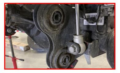
Make sure the frame is clear of debris before radius arm installation.
