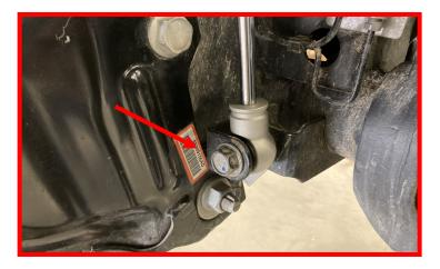
Remove the radius arm bolt at the frame on both sides.
