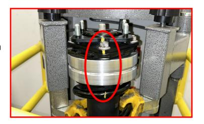
NOTE: During this process, ensure that the spring does not rotate relative to the lower spring perch.
