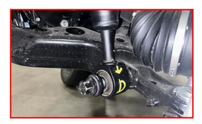
Install the tie rod into the knuckle.
