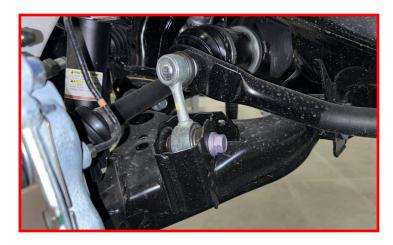
Put vehicle on ground. Tighten lower control arm bolts to 100 ft-lbs in order to get vehicle to alignment rack.
