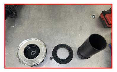
Install the isolator and dust boot into the top hat assembly. Preload spacer should be between the factory top hat and the isolator.
