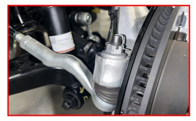
Install the sway bar end link to the lower control arm using factory hardware.
