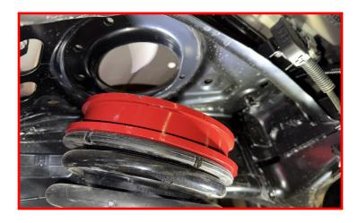
Ensure that the lower spring pigtail is in the correct orientation relative to the axle spring seat. The end of the pigtail should be against the ramped portion of the lower spring seat.
