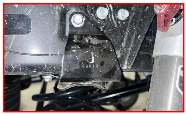
Install the supplied Falcon bump stop into the ReadyLIFT bump stop cup. Ensure that the bump stop is fully seated into the cup.
