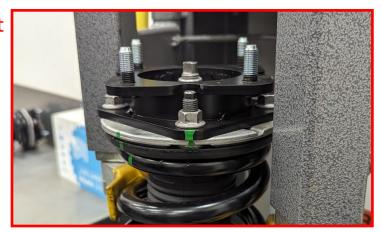
Compress the spring and carefully remove the top nut from the strut assembly.
