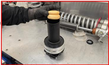
Install the top hat and preload spacer assembly. Rotate the top hat and ReadyLIFT front strut spacer so that the mark made in the earlier step aligns with the mark on the spring.
