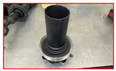
Install the bump stop into the dust boot in the orientation shown. Ensure that enough pressure is applied to set the bump stop into it's groove. The installation of the bump stop will also engage the retention feature of the dust boot.
