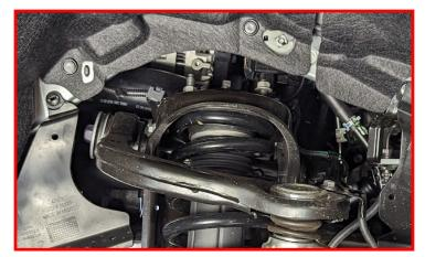
Slide lower strut off of the stud and remove strut from vehicle.
