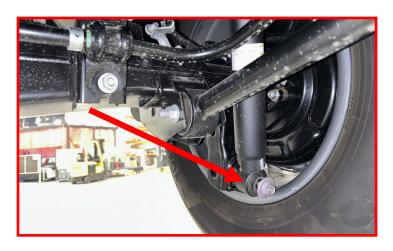
Install bolt into brake line bracket.
