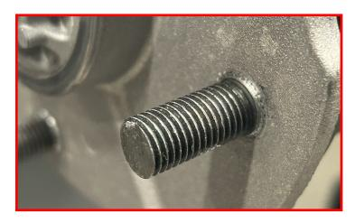
Install the ReadyLIFT front strut spacer onto the top of the strut. Torque nuts to 40 ft-lbs.
