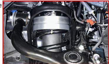
Replace the strut lower mount on the control arm stud and install the bolt.
