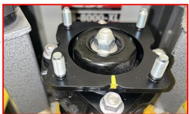
Remove the top hat, isolator, bump stop and dust boot from the strut assembly.
