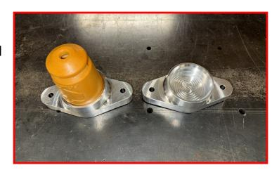
Apply some thread locker to the supplied M8 bolts and washers. Using these bolts and washers, install the ReadyLIFT Bump Stop extension and ReadyLIFT Bump Stop into the frame.
