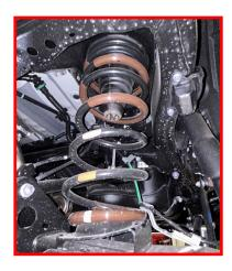
Install ReadyLIFT Spring Spacer on top of spring assembly. Retain factory isolator and ensure that the ReadyLIFT Spring Spacer is installed above the isolator.
