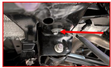
Install sway bar link into sway bar.
