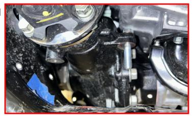
Assemble ReadyLIFT rear differential mount as shown.
