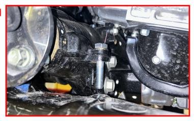
Raise the differential up to allow the install of the replacement diff drop.
