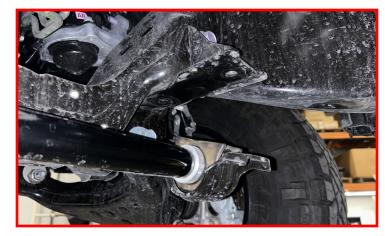
Install the core support nut.
