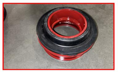
Install isolator and spacer onto the top of the factory spring.
