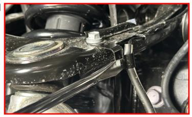
Remove the wire from the bracket.
