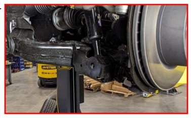
Install the factory lower shock bolt.
