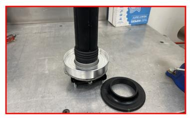
Install the spring isolator into the assembly.
