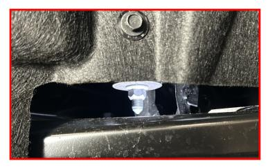
Install the inner fender liners.
