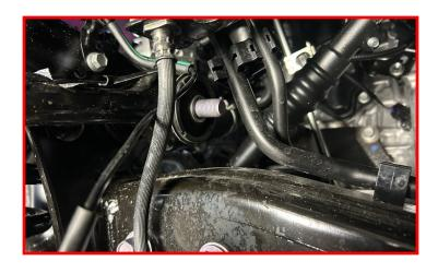
When removing the left (driver) side upper control arm pivot bolt, you will notice that the bolt will make contact with the intercooler/ boost tube.
