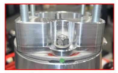
Install the completed strut assembly using the supplied M10-1.5 serrated flange nut.
