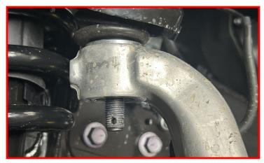
Remove the upper control arm pivot nut.
