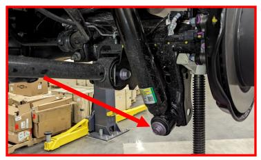
Loosen, but DO NOT REMOVE upper shock nut. Ensure axle is supported, and disconnect shock from axle stud. Remove shock from vehicle.
