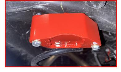
With the bump stop extension installed. Press the factory bump stop into the extension in a factory orientation.
