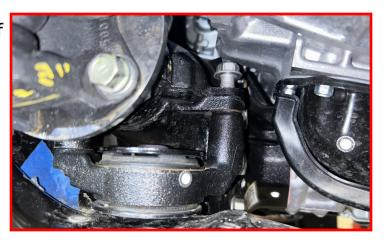
Raise the differential back up to allow the removal of the rear diff mount.
