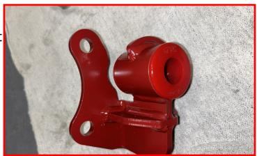
Install supplied crush sleeve through the bushing halves. Be sure to center the crush sleeve to the bushings.
