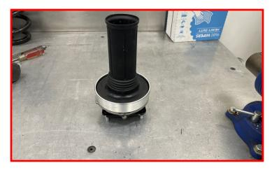
Install the top hat with the preload spacer, the isolator and the dust boot and rotate the top hat and ReadyLIFT front strut spacer so that the mark made in the previous step aligns with the mark on the spring.
