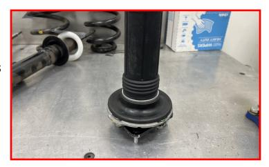
Install the ReadyLIFT preload spacer in between the top hat and the spring isolator. The lip of the preload spacer should be facing away from the top hat, (pointing down in vehicle).
