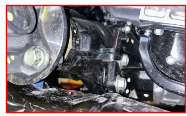
Install the supplied M12 x 60mm hex head bolt , washer and thread locker through the diff from top to bottom.
