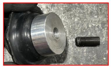
Install stud using internal hex.
