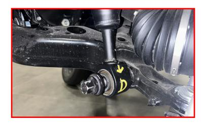
Install the tie rod into the knuckle.
