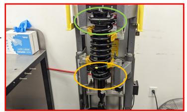
Make a mark on the ReadyLIFT front strut spacer, in line with the stud that is 45° counter clockwise from the mark made in the last step.
