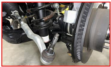
Remove lower control arm to strut bolt.
