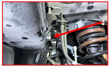
Install sway bar link into sway bar.
