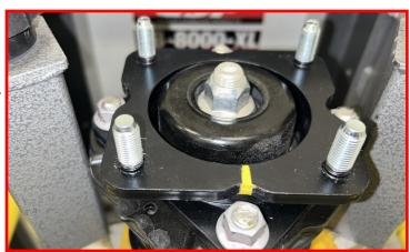
Remove the top hat, isolator and dust boot from the strut assembly.
