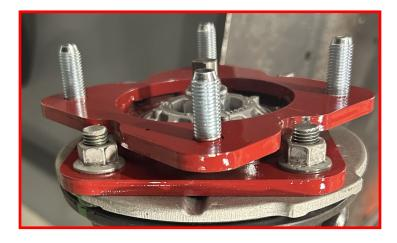
Place the strut assembly in a suitable spring compressor. The lower bushing hole should be perpendicular to your line of vision. Use a paint marker to mark relationship between the spring and top mount, as well as between the spring and bottom mount.
