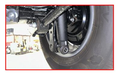
Remove headlight leveling link nut from axle bracket and let the headlight leveling link hang free.
