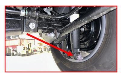
Install bolt into brake line bracket.
