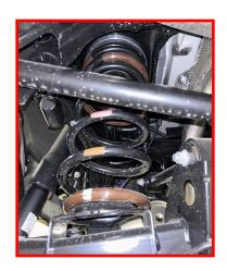
Ensure that the lower spring pigtail is in the correct orientation relative to the axle spring seat. The end of the pigtail should be against the ramped portion of the lower spring seat.
