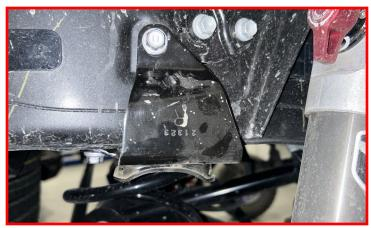
Apply some thread locker to the M8 bolts and washers. Using these bolts and washers, install the ReadyLIFT Bump Stop extension and ReadyLIFT Bump Stop into the frame.
