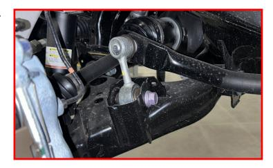
Put vehicle on ground. Tighten lower control arm bolts to 100 ft-lbs in order to get vehicle to alignment rack.
