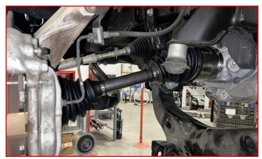
Install the supplied axle nut.
