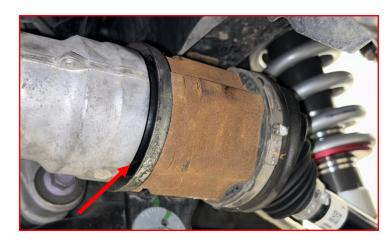
Remove the CV axle assembly from the vehicle.
