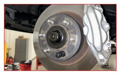
Remove the cotter pin and nut retainer.
