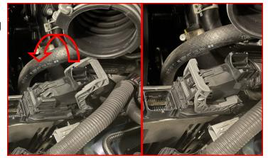
Plug the center plug into the accumulator and lock it in place by closing the handle to the right.
