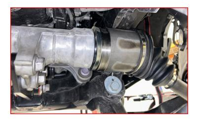
Install the outer splines through the hub assembly, in the factory orientation.
