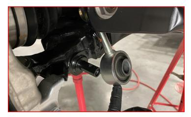
Remove the ABS wire bracket on the upper control arm.
