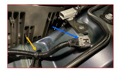
Release the leftmost accumulator plug by pressing in the tab and pulling the handle to the rear of the vehicle.
