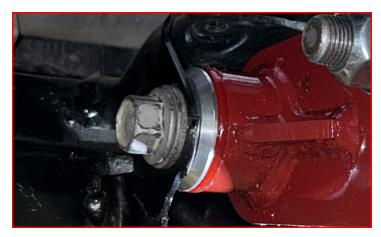
Install the factory bolts through the diff drop and diff drop bracket.
