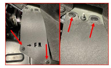
Remove the rear cover for caliper hanger hole.
