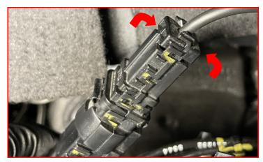
Slide the bracket into the plug housing until it clicks.
