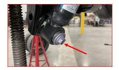
Remove the upper shock nut and bushing.
