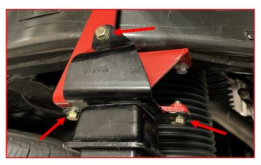
Install the rear brake line spacer—tall between the brake line and the axle using the supplied M8-1.25 x 40 flange bolt (one on each side) holding the brake line to the axle.
