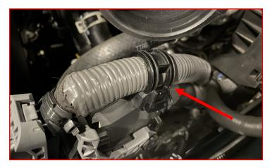
Plug the left most plug into the accumulator and lock it in place by closing the handle to the left.
