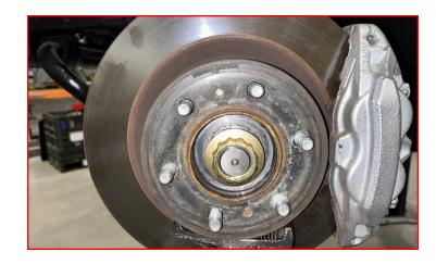
Install the nut retainer and supplied cotter pin.
