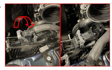
Clip the factory hose clip onto the wire housing for the center plug.
