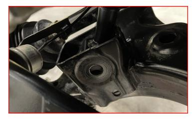
Remove the CV axle dust shield.
