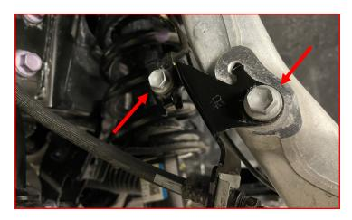
Using factory hardware, attach the ABS sensor wire at the bottom of the knuckle.
