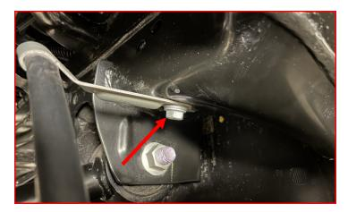
Remove the **bolt** holding the brake line to the frame.
