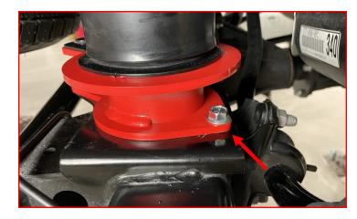
Use the supplied M10-1.25 serrated flange nut to attach it to the axle.
