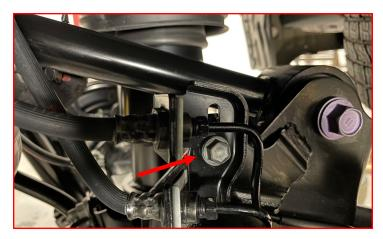
Install the end link onto the frame using factory hardware.
