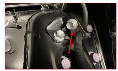
Remove both screws retaining the ABS wire to the middle of the knuckle.
