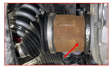
DO NOT TRY TO PRY THE AXLE FROM THE DIFF HOUSING, THIS WILL DAMGE THE HOUSING AND SEAL.
