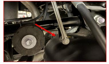
Using the supplied M6 bolt, washers, and locking nut, install the airbag ride height sensor bracket to the control arm with the bent location tab facing to the front of the vehicle.
