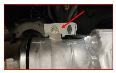
Relocate the bracket from the bottom on the mounting point to the top of the mounting point and attach using the factory hardware.
