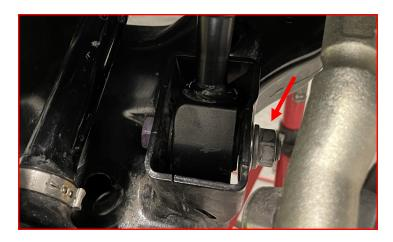
Raise the lower control arm enough to install the upper strut to the perch using the supplied M10-1.25 serrated flange nuts.
