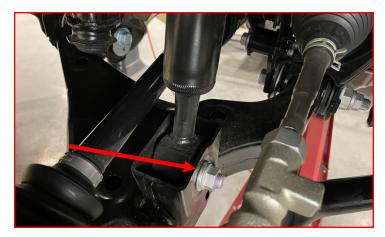
Remove the four (4) upper strut bolts.
