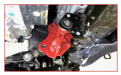
Install the supplied M14 x 55mm hex head bolt, flat washer and thread locker.
