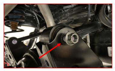
Remove the lower factory strut bushing from the shock.
