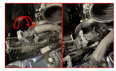
Clip the factory hose clip onto the wire housing for the center plug.
