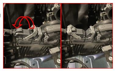
Plug the electrical plug back into its housing.
