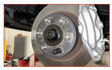
Remove the cotter pin and nut retainer.
