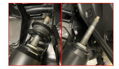
Apply a small amount of thread locker to the factory shock and install the ReadyLIFT rear strut extension onto the factory strut.
