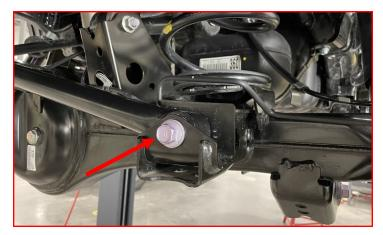
Loosen but **DO NOT** remove the **DRIVER** upper control nut at the axle.
