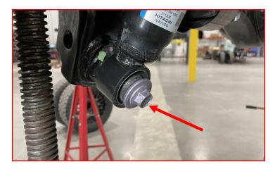
Remove the upper shock nut and bushing.
