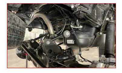
Place the ReadyLIFT rear spring spacer on the top of the factory bump stop and spring assembly as shown.
