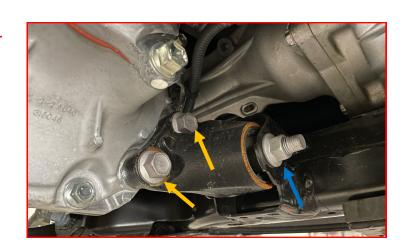
Above the passenger side bracket, the differential sensor wire needs to be relocated.
