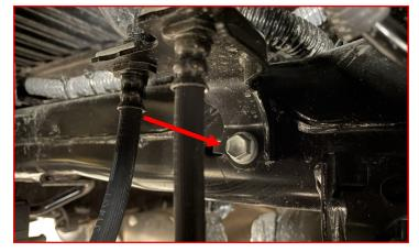
Remove the **bolt** holding the brake line to the axle.
