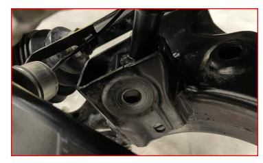
Remove the CV axle dust shield.
