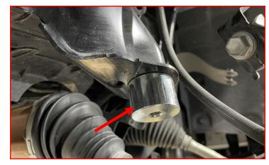
Attach the factory bump stop to the supplied extension.
