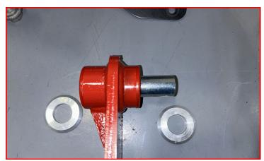
Install the front diff drop spacers on either side and ensure the large side of the spacer is touching the bushing.
