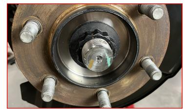
Remove the outer axle splines from the hub assembly.
