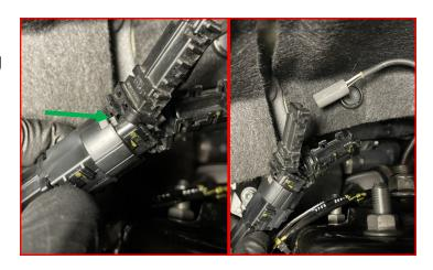
Using a trim removal tool, remove the four (4) clips for the plastic dirt shield.
