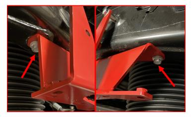
Attach the factory bump stop to the extension using the supplied M8-1.25 x 20 hex head bolts and M8 flat washers, starting with the lower bolts.
