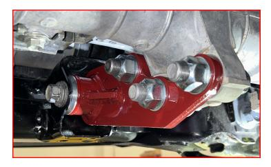
Torque the chassis to differential drop bracket hardware to 110 ft-lbs.
