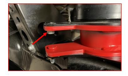
Remove the nut on the ride heigh sensor arm at the lower control arm.
