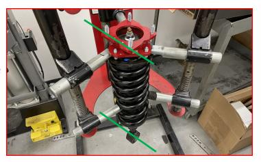
Carefully remove the strut from the spring compressor.
