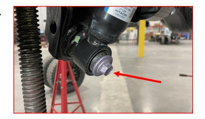
Remove the three bolts holding the factory bump stop to the frame.
