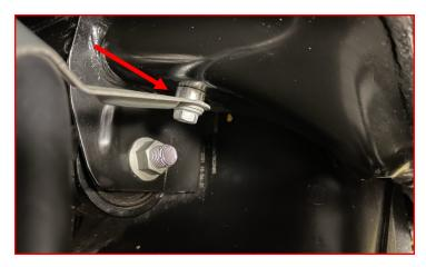
Using factory hardware, install the rear brake line relocation bracket holding the brake line to the frame.
