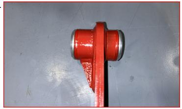
Install the diff drop into the frame side pocket in the factory orientation using the factory hardware.
