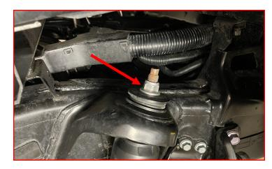
Compress the factory airbag enough to slide the supplied drill template between the airbag and the axle. Secure the template to the axle mount.
