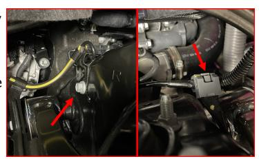
Using factory hardware, raise the lower control arm enough to install the lower strut bolt.
