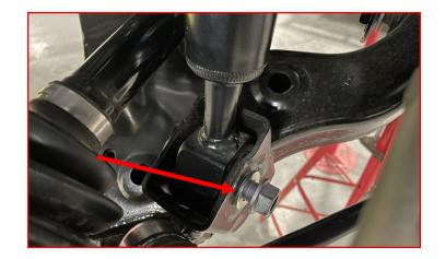
Apply a small amount of medium duty thread locker to the factory lower ball joint bolts.
