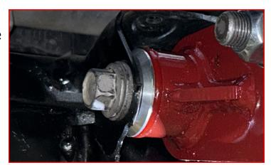
Install the factory bolts through the diff drop and diff drop bracket.
