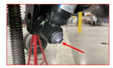
Remove the upper shock nut and bushing.
