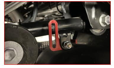
Attach the factory ride height sensor arm to the ReadyLIFT bracket using factory hardware.
