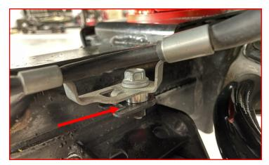
Install the rear brake line spacer between the brake line and the chassis using the factory bolt (one on each side) holding the brake line to the axle.
