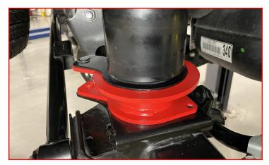
Insert the supplied M10-1.25 x 20mm flange bolt and M10-1.25 flange nut into the previously drilled hole.
