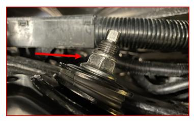
Torque the lower shock bolt to 60 ft-lbs.
