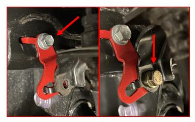
Install the bracket holding the brake line to the axle using factory hardware.
