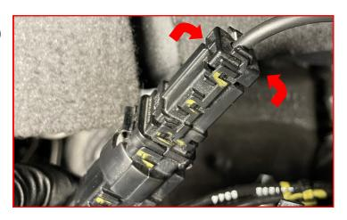
Slide the bracket into the plug housing until it clicks.
