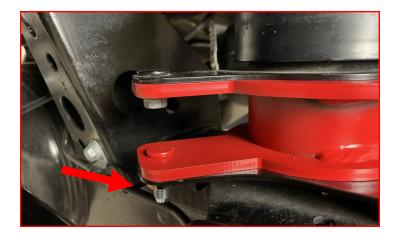
Use the supplied M8-1.25 extended thread nut to attach the airbag to the spacer.
