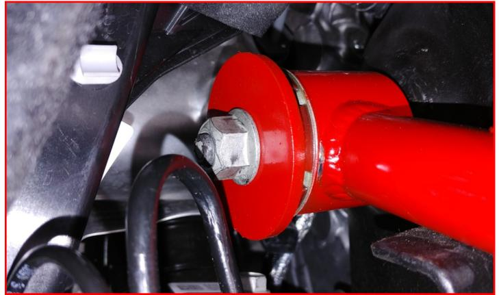
Once upper control arms have been properly torqued, install the supplied **top strut spacer** on the top of the strut assembly. Install completed strut assembly into the vehicle using the supplied **M10 serrated flange nuts**.
