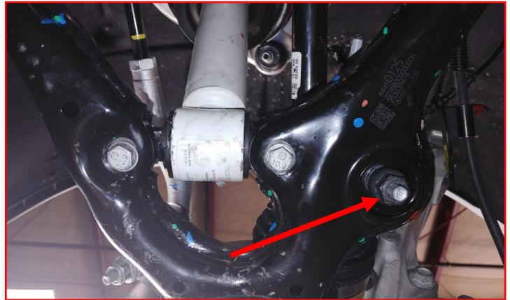
Remove the **CV axle nut**. Press axle back through hub to allow for greater misalignment and ease in the removal/installation process.
