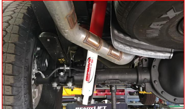
Remove the driver side U-bolts completely and discard. Lower the axle enough to remove the factory lift block making sure that all brake lines and ABS lines do not get over extended.
