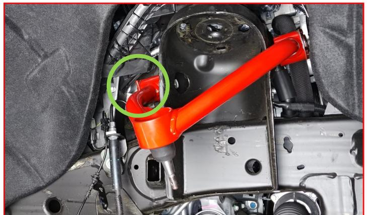
With the upper control arm bolts in place, install the supplied **laser cut washers**, the **factory nuts** and a drop of **thread locker**.
