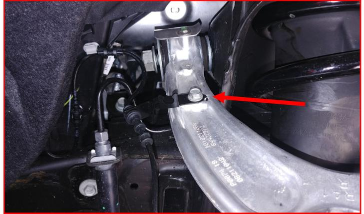
Remove the **lower sway bar end link** from the lower control arm. Retain factory hardware.
