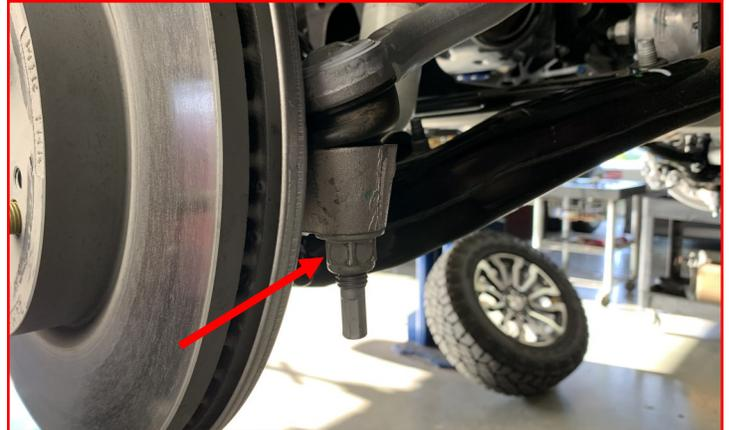
Install the **ABS sensor harness and brake-line bracket** to the knuckle.
