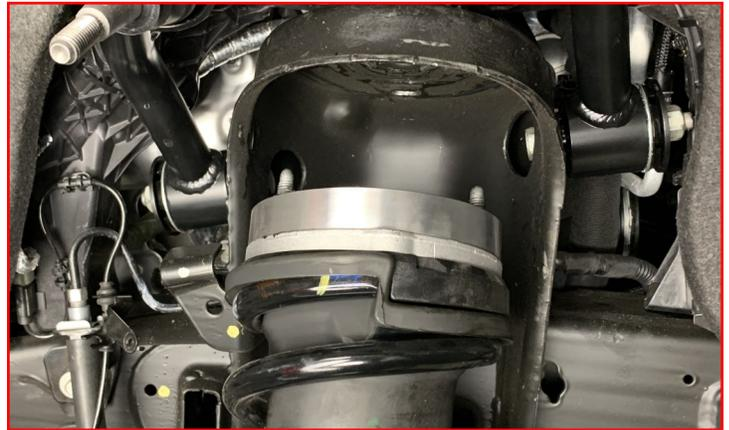
Install the factory lower strut bolts.
