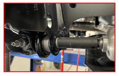
Torque the factory end link hardware to 35 ft-lb.
