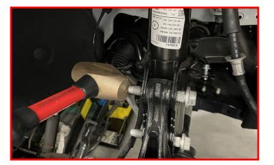
Support/ hold the strut to prevent it from falling and remove the 13mm upper strut bolts from the engine bay.
