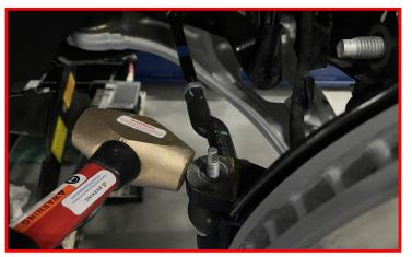
Remove and discard the factory end link from the vehicle using an 18mm socket/ wrench and a T40 Torx bit.
