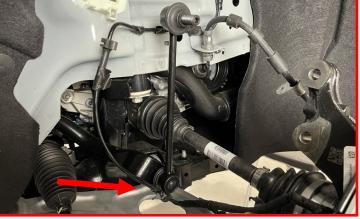
Using a sanding disk, grind down the inboard edge on the bottom of the strut so it's flush with the strut body.
