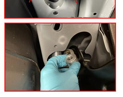
Bolt in the trailing arm using the supplied M14-2.0x60mm bolts, M14 flat washer, and lock washer.
