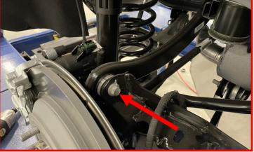
Loosen, but **DO NOT REMOVE**, the rear trailing arm 15mm bolt.
