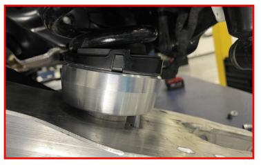
Using a jack, carefully lift the lower control arm until the factory strut bolt and lock nut can be installed.
