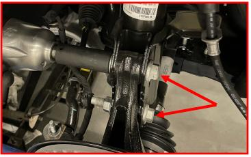
Use a hammer to remove the bolts from the knuckle.
