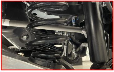
Carefully use a prybar or flathead screwdriver to remove the spring isolator from the lower control arm.
