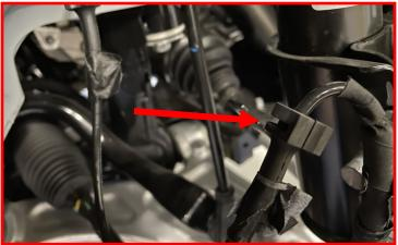
Use a trim removal tool to remove the ABS wire clip from the knuckle.
