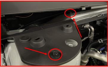
Remove the 21mm lower strut nuts on the knuckle.
