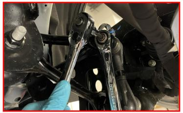
Return sound dampening liner to its original position. Reinstall the factory nut and trim clip.
