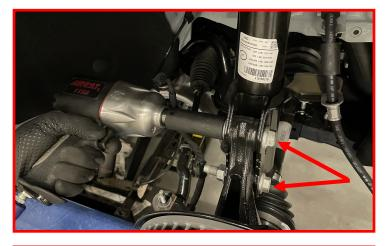
Mount the End Link to the End Link Drop Bracket using the supplied hardware.
