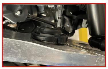
To access the trailing arm bolts, lower the sound dampening liner by removing the 10mm nut and trim clip towards the rear of the vehicle.
