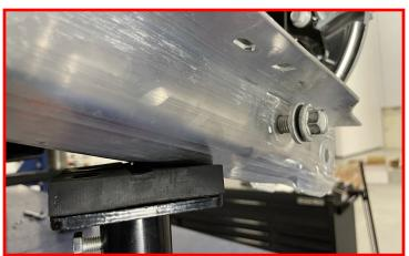
Continue to carefully lift the lower control arm until the factory lower knuckle bolt and lock nut can be installed. Be careful to not lift the vehicle off of the jack stands/ lift.
