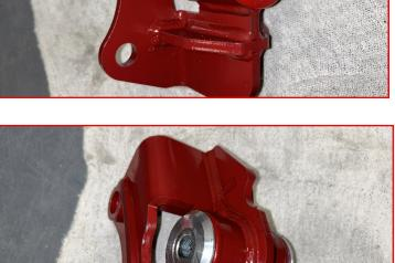
Install the diff drop into the frame side pocket in the factory orientation using the factory hardware.
