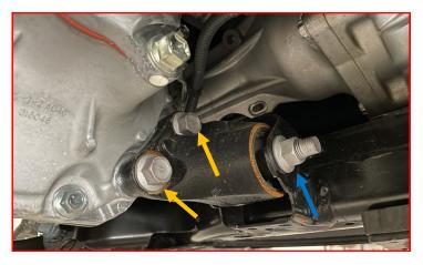
Above the passenger side bracket, the differential sensor wire needs to be relocated.
