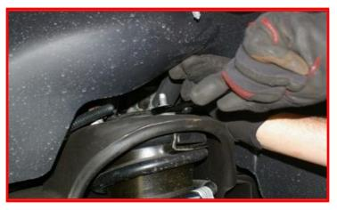
Remove the strut from the vehicle.
