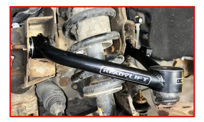
Install the strut starting with the upper mount nuts.
