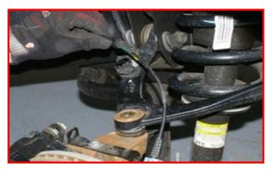
Remove the brake line bracket from the upper control arm and frame rail.
