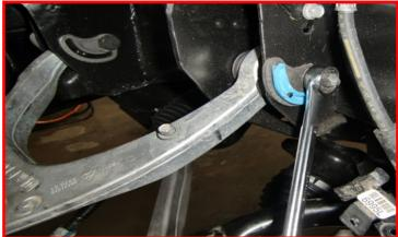
Install the appropriate side replacement upper control arms into the frame using the previously removed cam bolts and cams.
