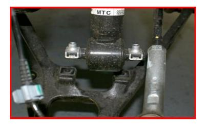
Remove the upper strut mount nuts at the frame.
