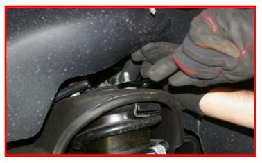
Remove the strut from the vehicle.
