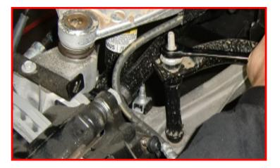
Remove the axle nut at the hub bearing. This is to keep the CV axle from being over extended when lowering the control arm in a later step. You may have to remove a axle nut cover to access this nut.
