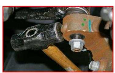
Unbolt the strut from the lower control arm.
