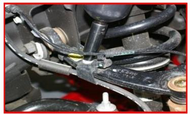
Remove the sway bar end links from the sway bar and lower control arm.
