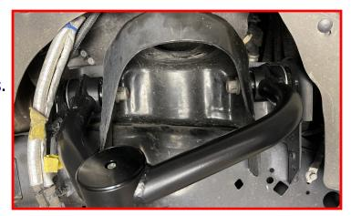
Install the ball joint into the knuckle.
