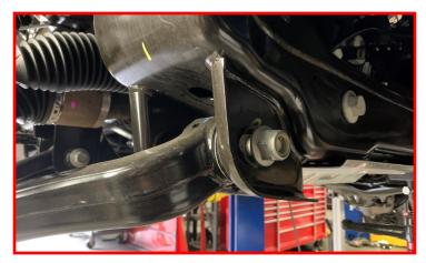
Tighten the top strut nuts.
