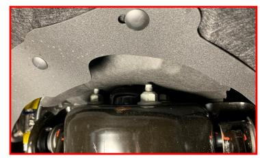
Remove the lower strut nuts.
