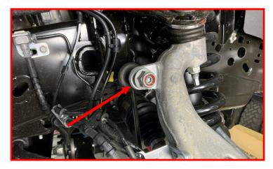
With everything tightened and torque to the specified specifications, install front tires and lower vehicle. Torque the lower control arm hardware to 200 ft-lbs
