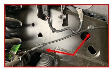
Connect the CCD solenoid harness connector.
