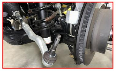
Remove lower control arm to strut bolt.
