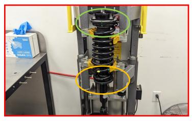
Make a mark on the ReadyLIFT front strut spacer, in line with the stud that is 45° counter clockwise from the mark made in the last step.
