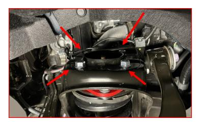
Using factory hardware, rise the lower control arm enough to install the lower strut bolt.
