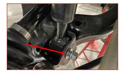
Apply a small amount of medium duty thread locker to the factory lower ball ioint bolts.
