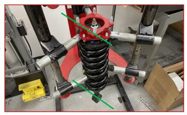
Carefully remove the strut from the spring compressor.
