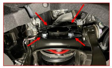
Tighten inner control arm hardware. Final torque spec should be set by alignment technician.
