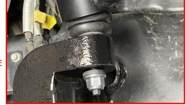
Install the supplied adel clamp on the front tube of the upper arm.
