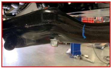
Using an appropriate jack, carefully jack the lower control arm into the frame side pivot pockets. Install the factory pivot bolts.
