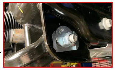
Tighten the top strut nuts.
