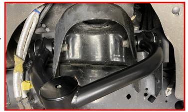
Install the ball joint into the knuckle.
