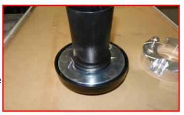
Install the factory nuts onto the strut hat studs running them down until they bottom out. Using a suitable cutting tool, cut the studs off just above the nut. Remove the nuts and clean any off any burrs. Paint the exposed metal with a quality rust preventative paint.
