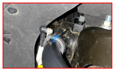
Using the factory nuts, install the completed strut assembly into the frame.
