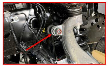
Complete all installation steps on the opposite side. Torque the lug nuts to the wheel manufacturers specs and lower the vehicle. Jounce the vehicle to settle the suspension to the new ride height. Torque the lower control arm hardware to 200 ft-lbs.
