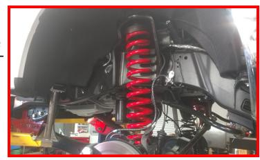
Install the Falcon Front Shock using the provided hardware on the top and the factory hardware on the bottom attachment. Torque the upper shock hardware to 35 ft -lbs. Leave the bottom shock hardware loose at this time.
