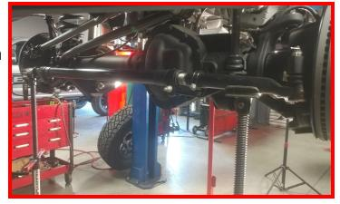
Remove the bolt from the rear pivot of the factory radius arm. Retain factory hardware.
