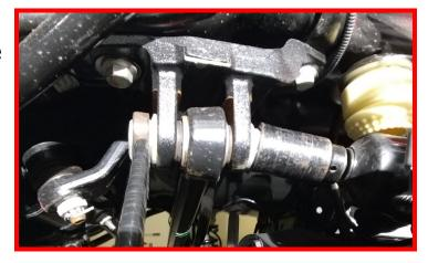
Remove factory track bar bracket and discard. Using the factory hardware, install the supplied track bar bracket on the frame in the factory orientation.
