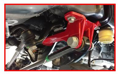
Install the ReadyLIFT sway bar drops to the frame using factory hardware. Torque to 35 ft-lbs. Install the sway bar to the ReadyLIFT sway bar drops using the 7/16" x 1 1/2" bolts, washers and nuts. Torque to 35 ft-lbs.
