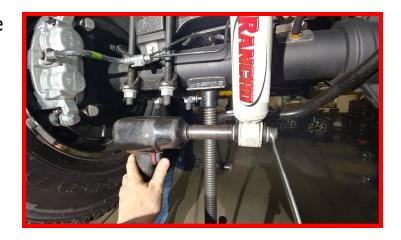
Slightly loosen but do not remove the passenger side u-bolts. Remove the driver side u-bolts completely and discard.
