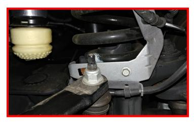
Remove the factory bump stop by pulling it out of its mount. Remove the mount from the frame.
