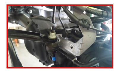
Support the axle with a suitable jack and remove the lower shock hardware from the axle mount. Retain factory hardware.
