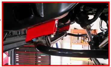
Install the ReadyLIFT brake line bracket to the factory brake line using 5/16" x 3/4" bolts, washers, and nuts. Install the bolt facing outwards. Torque to 10 ft-lbs. Gently pull the metal brake line down while lining up the ReadyLIFT bracket to the original holes in the frame. Install using factory hardware. Torque to 5 ft-lbs.
