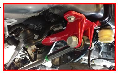
Lower the axle enough to remove the front springs. Install the replacement spring using factory rubber isolator. Raise the axle enough to hold the spring assembly in place.
