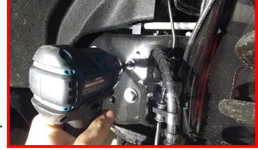
Remove the brake line bracket at the axle. Retain the factory hardware.
