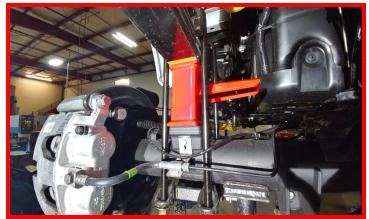
Install rear Falcon shock using factory hardware.
