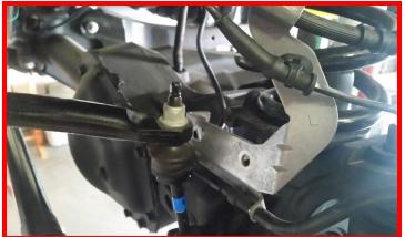
Support the axle with a suitable jack and remove the lower shock hardware from the axle mount.
