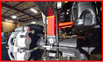
Install rear Falcon shock using factory hardware.
