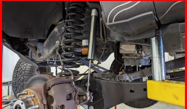
Remove the jack stands from under the axle and let the axle hang. Place those jack stands under the tie rods as shown in the image.
