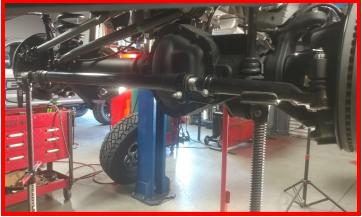
Remove the factory radius arm pivot hardware.
