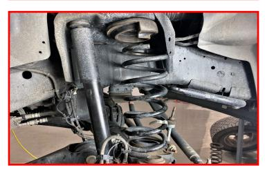
Remove the factory spring isolator.
