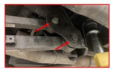
Loosen the axle side control arm bolts.
