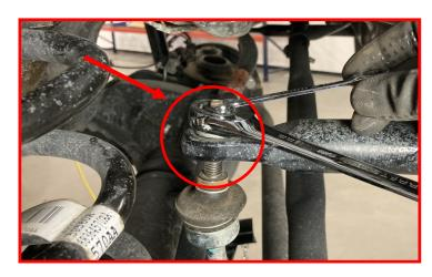
Reinstall the 13mm lower ABS and Brake line bracket bolt located on the axle.
