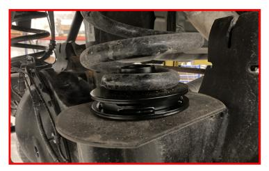
Install the shock shaft in the frame side factory shock location.
