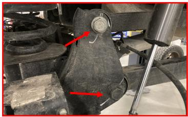
Loosen the rear track bar at the frame side.
