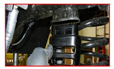
Using thread locker install the (3) supplied 5/16" bolt from the inside out on the supplied spring isolator retainer.
