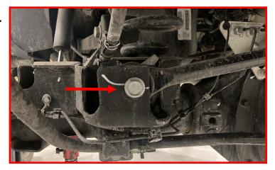
Remove the factory rear shocks upper and lower mounting hardware.
