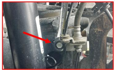
Remove the 18mm nut from the sway bar end link while holding the 8mm bolt so it does not spin.
