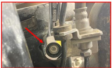
Install the 13mm upper ABS and Brake line bracket bolt located above the radius arm.
