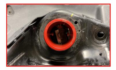
Place the spring isolator onto the provided lift springs and install the provided spring.
