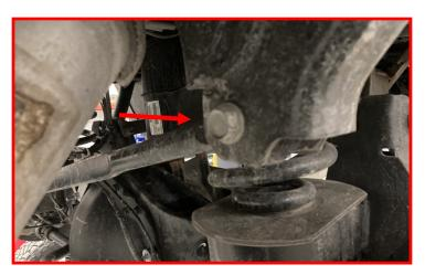
Loosen the rear track bar at the axle side.
