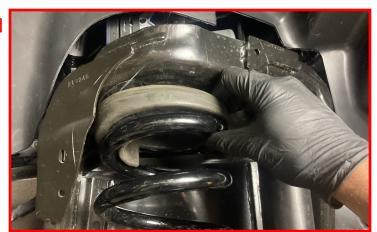
Make sure to align the end of the coil to the corner of the axle's spring perch to maintain the correct spring position.
