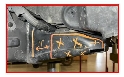
Using an appropriate tool and taking proper safety precautions, cut along the lines that were drawn in the previous step. Take extra care not to cut into the body mount bushing or any other critical components.
