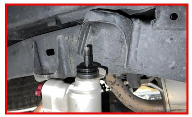
Install the shock onto the lower shock mount on the axle.
