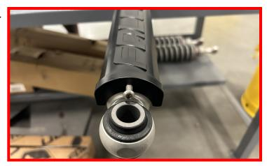
Install Falcon Rear Shock alignment tab below the bushings of the shock. The longer alignment tab will be used on the driver's side, while the shorter one is for the passenger side.
