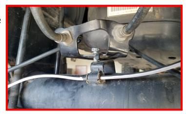
Remove the emergency brake line bracket bolt.
