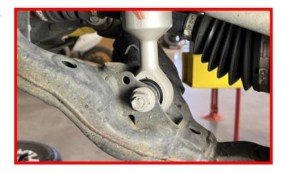
Install the lower ball joint cradle to the knuckle using the factory hardware, and a drop of thread locker.
