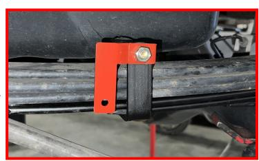
Install the center pin through the Ready-LIFT Mini Pack and the factory leaf springs.
