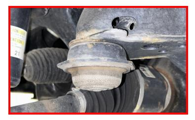
Apply a small amount of thread locker to the threads on the bump stop. Install the provided front bump stop spacer and reinstall the Bump stop.
