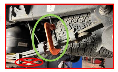
Once firmly clamped on each side, remove the center pin and overload spring and discard those items.
