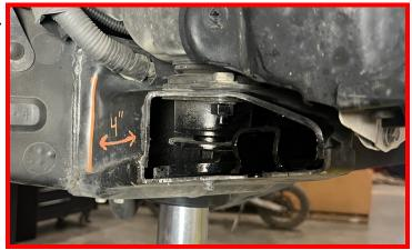
Use an appropriate tool to clean the area around the cut of any paint or debris.
