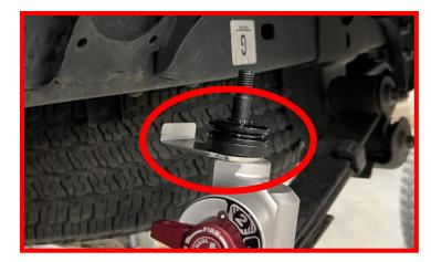
Install the Falcon rear shock into the upper shock mount on the frame. The alignment tab should be pointing toward the frame. Install the upper bushing and nut.
