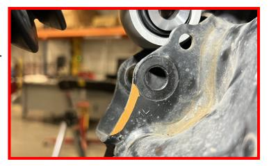
Using an appropriate tool, cut away the marked material. Ensure the cut surface is smooth and free of burrs. Paint the cut surface with an appropriately rated coating in order to avoid rust.
