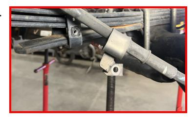
Support both sides of the axle with adjustable jacks.
