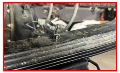
Install the Falcon pump stop into it's cup, ensuring that it is fully seated, and place the assembly onto the leaf spring, lining it up with the center pin. The wings of the unit should be parallel with the leaf spring.
