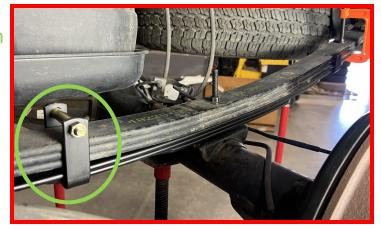
Install the brake line bracket onto the horseshoe, with the L shape pointing forward and down. Ensure that the metal crush sleeve on the horseshoe bolt is retained.
