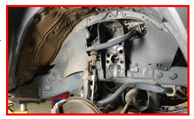
On the rearward side of the lower strut mount on the lower control arm, it will be necessary to trim the material marked in yellow. Make the same mark on each lower control arm. This will allow for proper clearance with the CV boot.
