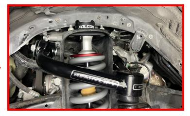
Install the ball joint into the knuckle using the provided nut and laser cut washer.
