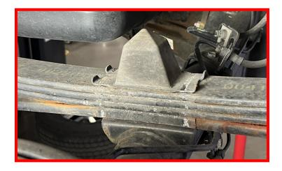
Clamp the front portion of the leaf spring using a heavy-duty metal clamp. Ensure that all leaves of the spring are clamped, less the overload spring. Clamp should be placed as far forward on the spring as possible while still capturing each leaf.
