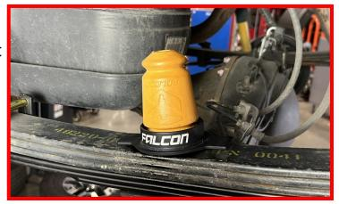
Install the factory U-bolts. Ensure that the U-bolts go over the wings of the Falcon Bump Stop, securing it to the top of the leaf spring.
