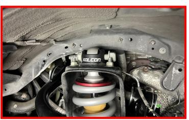
Install lower strut bushing into the lower control arm using factory hardware.
