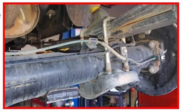
Remove the u-bolts of the side you are working on.
