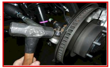
Support the hub assembly with an appropriate jack. Remove the lower strut hardware.
