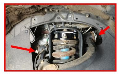
Install the ReadyLIFT upper control arm using the factory upper control arm pivot bolt and nut. Remove upper control arm from vehicle.
