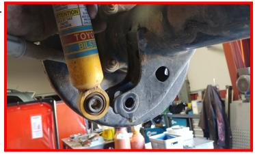
Remove the rear shock from the frame mount. Shock and hardware can be discarded.
