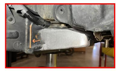
Using an appropriate paint for automotive frames, paint the surface thoroughly.
