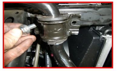
Install the ReadyLIFT sway bar brackets to the frame using the factory hardware.
