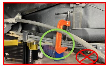
Repeat the process on the rear of the spring, again ensuring that all leaves of the spring are clamped, less the overload spring.
