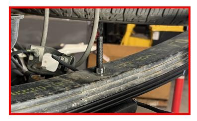
Trim off the excess length of the center pin so that it is almost flush with the top of the nut. It shouldn't be completely flush, two threads should be sticking up from the top of the nut.
