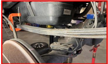
Install the ReadyLIFT Mini Pack so that the horseshoe with the bolt going through it is pointed toward the front of the vehicle.
