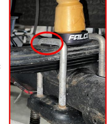
Install the factory bottom plate and U-Bolt nuts.
