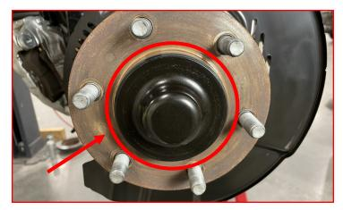
Remove the cotter pin, sleeve, and nut.
