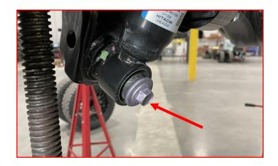
Remove the upper shock nut and bushing.
