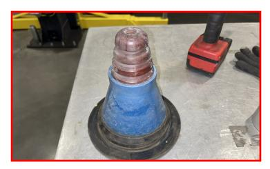
Secure the ReadyLift bump stop extension to the plastic holder using the supplied M10 Bolt and Washer.
