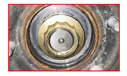
Slide the factory axle nut cover on.
