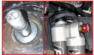
Slide the rear shock over the shock mount and secure using the factory hardware.
