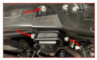
Install the ReadyLift bump stop and bump stop extension using the supplied M8-70mm bolts and washers.
