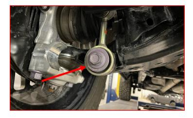
Torque the sway bar bracket factory hardware to 80 ft-lbs.
