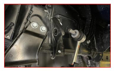
Remove the Panhard bar bolt at the axle and let it rest in the mounting perch.
