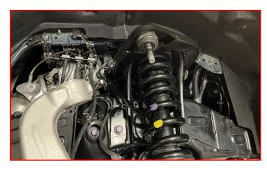
Support the CV axle to prevent damage
