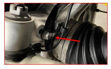
Start the two supplied M8 bolts and washers in the rear crossmember. Leave them loose to slide the slotted holes on the skid plate into place.
