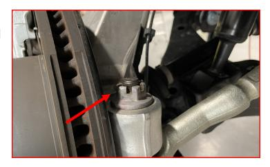
Remove the CV axle dust shield.
