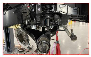
Remove the lower shock bolt, let the lower control arm hang out of the way.
