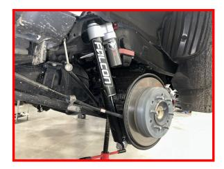
Bolt the shock alignment tab to the frame using the provided hardware.
