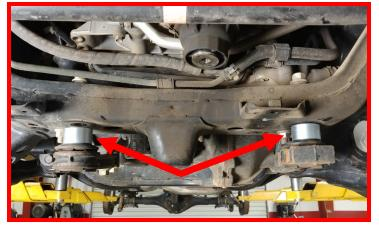
Attach differential brackets with provided hardware. Use factory large bushing washers in their original location.
