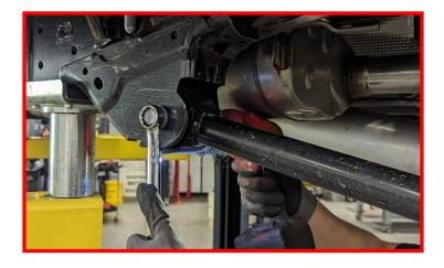
Disconnect sway bar link from the frame on both the left and right hand sides.
