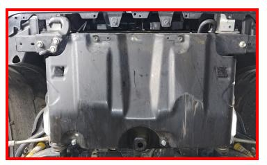
Install the rear of the front gravel guard using the provided M8 x 40mm hardware and spacers. Torque front and rear hardware to 5 ft-lbs.
