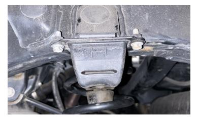
Install the ReadyLIFT Bump Stop Spacer using the provided M8 bolts and washers.
