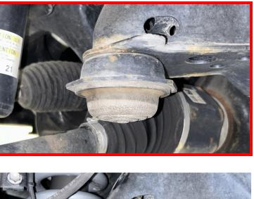
Apply a small amount of thread locker to the threads on the bump stop. Install the provided front bump stop spacer and reinstall the Bump stop.
