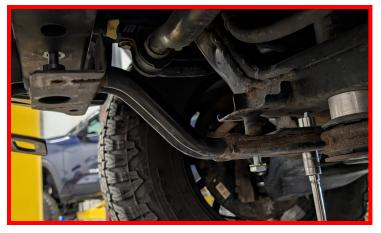
Install the jack point spacer to the front gravel guard using the provided M8 Bolts and washers.
