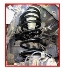
Falcon rear shock is provided with dust shield and alignment tab.
