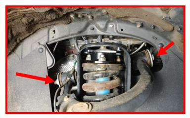
Install the ReadyLIFT upper control arm using the factory upper control arm pivot bolt and nut. Remove upper control arm from vehicle.
