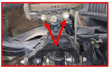
Reconnect the tie rod to the steering knuckle using factory hardware.
