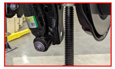
Ensure axle is supported and remove upper shock nut. Remove shock from vehicle.
