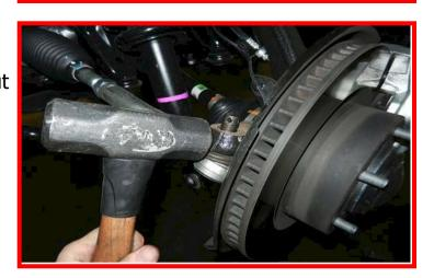
Support the hub assembly with an appropriate jack. Remove the lower strut hardware.
