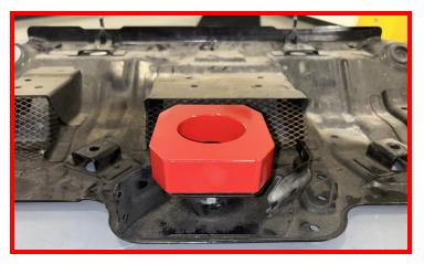
Install the front two bolts of the front gravel guard to the core support cross member using the factory hardware.
