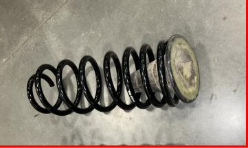
Install ReadyLIFT Spring with factory isolator into the vehicle.
