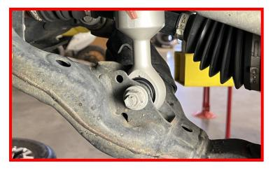
Install the lower ball joint cradle to the knuckle using the factory hardware, and a drop of thread locker.
