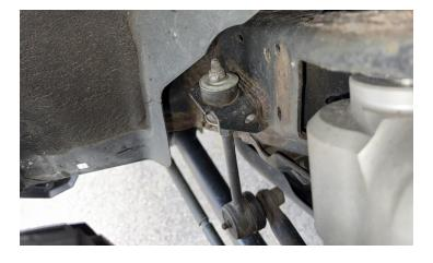
Prior to installing wheels, complete all installation steps on the opposite side. Install the wheels and lower the vehicle to the ground. Torque the lug nuts to the wheel manufacturers specs. Jounce the vehicle to settle the suspension to the new ride height. Torque all rear control arm hardware to 135 ft-lbs.
