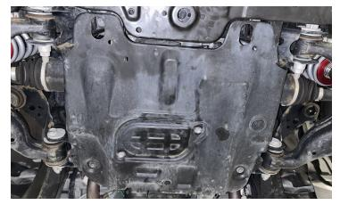
Remove front differential mounts from the frame and let it hang. Retain large bushing washers.
