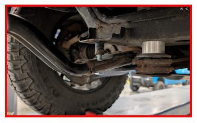
Install the other two spacers and bolts into the support bracket.
