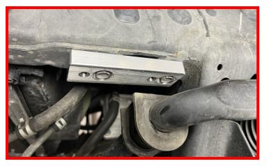
Install the sway bar to the ReadyLIFT brackets using the provided M10 x 20mm bolt and washer.
