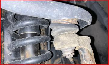
Remove the upper control arm pivot bolt and nut. Remove upper control arm from vehicle.
