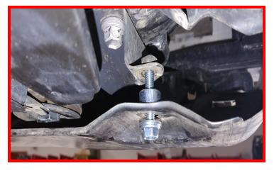
Install the ReadyLIFT skid plate using the factory bolts in the front, and the provided M8 bolts in the rear.
