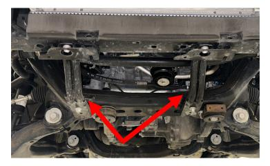
Using the provided spacer and M10 hardware, install the middle bolt of the front support bracket. The spacer will be installed inside the pocket of the support bracket.
