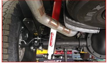
Remove the driver side u-bolts completely and discard. Lower the axle enough to remove the factory lift block making sure that no brake lines or ABS lines get over extended.
