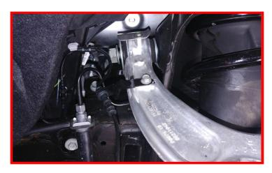
Use the supplied zip ties to secure the ABS wire to the tab on the control arm.
