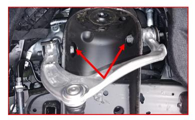
Bend **ASSEMBLY TAB** on frame slightly inward to allow clearance for the added down travel of the suspension.
