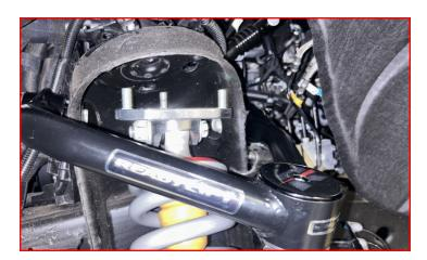
Install supplied M10 bolts through Falcon cross pin and lower control arm. Install M10 washers, and nuts.
