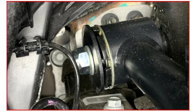
Attache the top hat to the coilover using the supplied M16 hardware. Torque to 180 ft-lbs.
