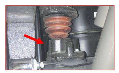
If the truck DOES NOT HAVE the 2" cast bump stop extension shown in the previous picture, INSTALL THE READYLIFT BUMPSTOP EXTENSION as follows.
