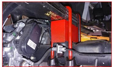
Install the Falcon shocks using the factory hardware as shown.
