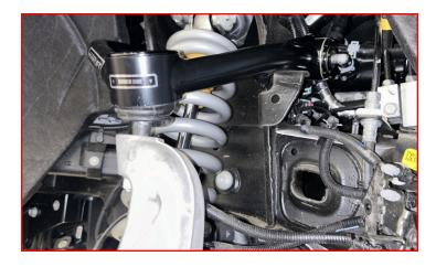
Torque the axle nut to 160-ft/lbs.
