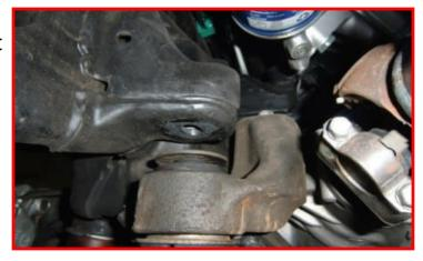
Install the two rear 1/2" ReadyLIFT differential spacers between the frame and differential cradle followed by the front. Use the provided M14 washers and M14x130 bolts, reuse factory flange nuts.
