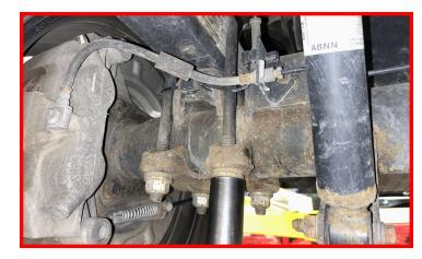
Lower the axle down enough to install the ReadyLIFT block on the driver side.
