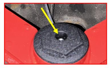
Install Falcon front shock using supplied hardware on top and factory hardware on the bottom.
