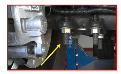
Install the Falcon rear shocks (reservoirs down) using the factory hardware.
