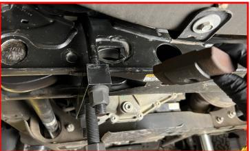
Standard model torsion bar reuse factory torsion arm adjustment bolt.
