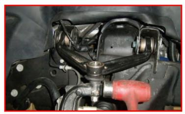
Remove the upper control arm bolts from the frame rails. Mark the cam bolt and cam orientation for re-installation.
