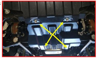
Locate the four (4) front and rear differential cradle bolts. Loosen but do not remove all four and lower the differential.
