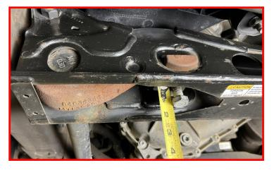
Using a torsion bar unloading tool (ReadyLIFT part #66-7816A), relieve the pressure on the torsion key cross pin.
