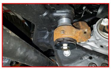
Install the differential skid plate with the rear mount only at this time. Insert the 1/2" spacers between the crossmember and skid plate. Use the supplied M10x40mm bolts and M10 fender washers.
