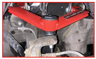
Grease the upper ball joint using a high quality ball joint grease and a needle type grease gun. DO NOT over grease.
