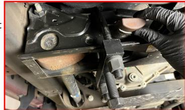
Push the torsion bar forward through the factory keyway cross member and lower control arm. You may need to use a hammer and punch on the end of the bar to break it loose from the keyway and control arm. Remove the torsion bar key.
