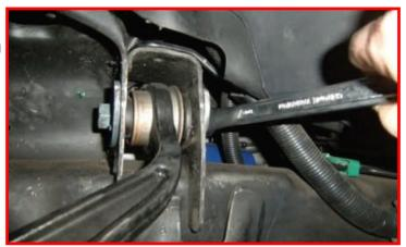
Remove the upper control arm from the frame rail.
