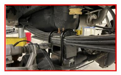
Install the rear sensor bracket on the forward axle center pin in the factory orientation.
