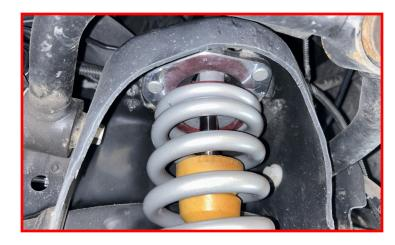
Install the provided M16 Flange bolt through the top hat and coilover from front to rear.
