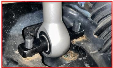
Install the supplied M12 lower strut nuts.
