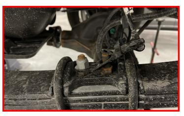
NOTE: WHEN UNBOXING THE FALCON REAR SHOCK, YOU'LL NOTICE THE LOW-ER RODENDS MAY BE ORIENTATED DIFFERENTLY. IT IS EXTREMELY INPORTANT THAT ROD END IS ORIENTED TO THE (3) MOUNTING HOLES FACE THE OPPOSITE DIRECTION OF THE RESERVOIR.
