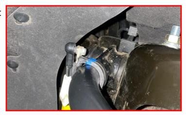
Install the coilover top hat adaptor plate, using the supplied thread locker and M10 flanged head bolts. Ensure the Falcon logo is facing out towards the wheel.
