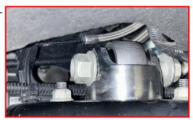
Continue to raise the lower control arm up until you are able to install the supplied M12 bolts and washers.
