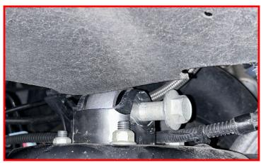
Install supplied M16 locking flange nut onto the coilover mounting bolt.
