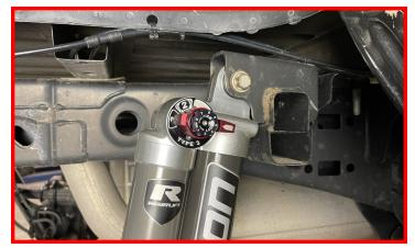
Install the lower shock bushing into the axle perch using the factory mounting hardware.
