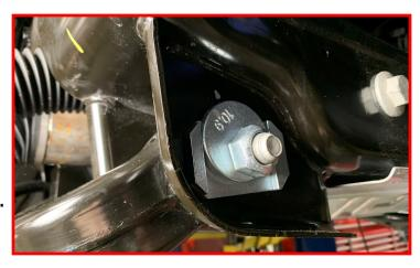
Tighten the top strut nuts.
