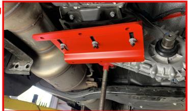
Ensure that the mount is installed with the slope facing towards the rear of the vehicle.
