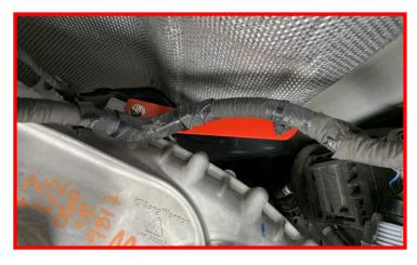
Install the transfer case shift solenoid connector.
