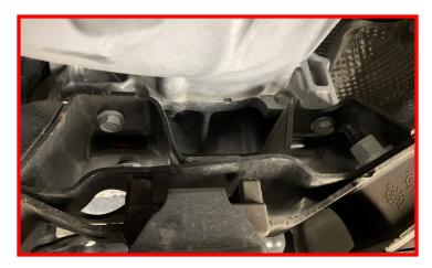
Tighten the transmission mount bolts.
