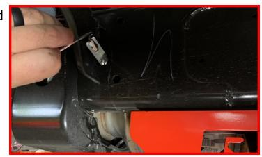
Once lined up with the lower mounting holes, install the provided 1/2" bolts and washers.
