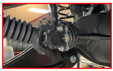
Rotate the axle to release radius arms from the mounting locations.
