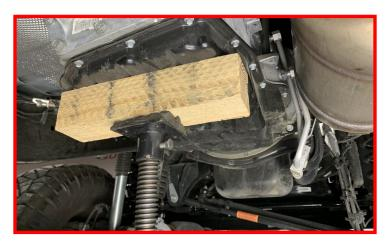
Ensure the transfer case is free of any other harness clips and the harnesses are not wrapped, hung on or caught on any part of the transfer case.
