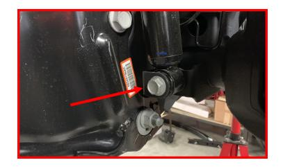
Place a jack under the axle for support. Remove the radius arm bolts.
