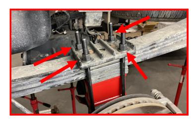
Install the provided rear brake line bracket extension using the upper slots to the factory bracket using the provided M8 hardware. Torque provided hardware to 20 ft-lbs.
