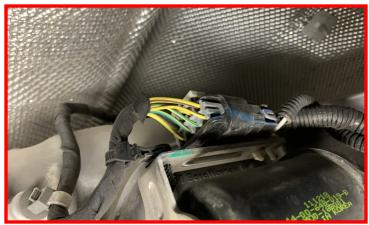
Install the transfer case harness retaining clip on the rear of the transfer case.
