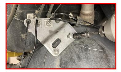
Remove the clips on the back side of the axle that secure the brake lines.
