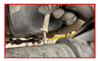
Remove the brake line brackets under each leaf spring.
