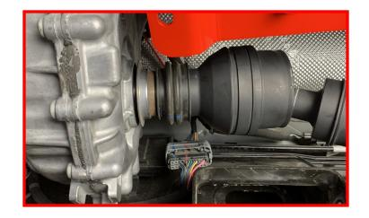
Install the provided clamp onto the dust boot and joint housing.
