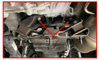
The remaining (2) bolts are located at the front of the mount. Remove the (2) bolts and remove the mount.
