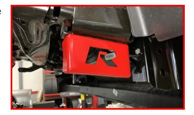
Install the sway bar to the drop brackets using the provided 7/16" hardware.
