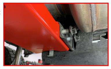
Install (3) provided M12 bolts, (3) locking nuts and, (6) flat washers through the rear holes on the transmission mounting plate, mounting plate spacer and the transmission crossmember.
