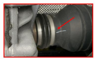
Using the appropriate pliers, spread open the retaining clip and slide the front driveline off the splines.
