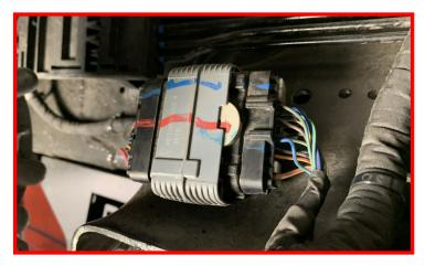
With the connector out of the way, install the connector relocation bracket using the provided M6 hardware.
