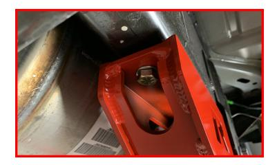
Bend the wires to align the tab nut with the front mounting holes in the bracket and frame. Install the provided 1/2" bolts and washers.
