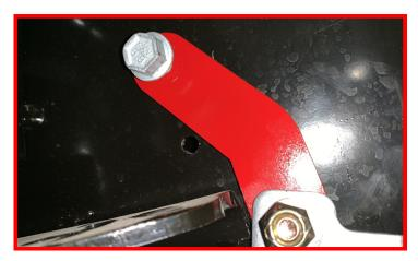
Install the ABS sensor harness and brake line bracket to the radius arm using factory hardware.
