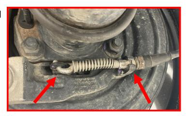
Tighten the e-brake adjustment bolt until you have the correct tension on the cable.
