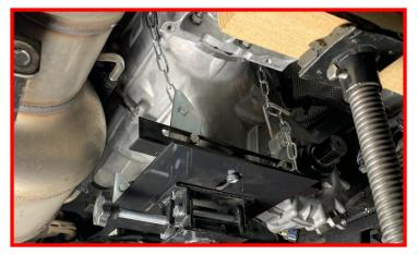
Remove the (8) transfer case mounting nuts.
