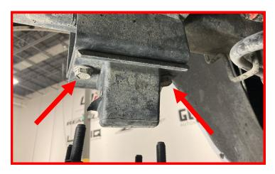
Install the bump stop extension onto the frame using factory hardware.
