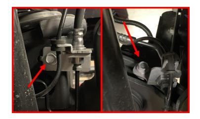
Locate the brake line/ABS bracket on the inside of the driver and passenger frame rails and remove.
