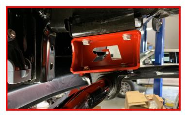
Install provided brake line extensions to the frame brake line brackets using the provided 5/16" hardware. Do not tighten at this time.
