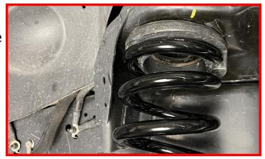
Install front shocks using factory lower hardware and provided upper hardware.
