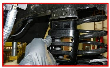
Using the supplied drill template, align the corresponding hole with the correct side. "D" will line up with the factory driver side hole and the "P" will line up with the passenger side hole.
