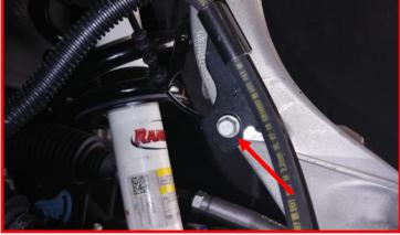
Remove the ABS sensor harness bracket from the knuckle.
