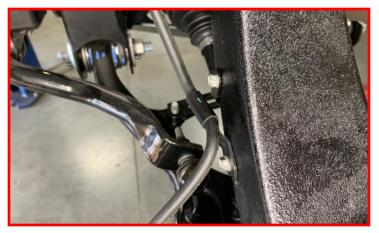
Using wire ties, secure the ABS sensor harness to the brake line.
