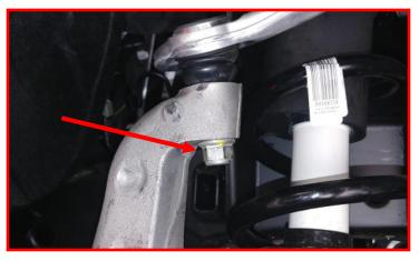
Support the lower control arm with a suitable jack. Remove the lower strut mounting bolts from the lower control arm.
