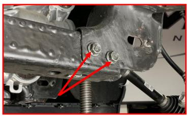
Remove passenger side differential mounting hardware.
