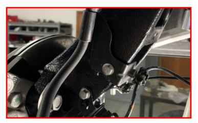
Install ABS sensor harness/ brake pad sensor bracket to the inside of knuckle. It is necessary to remove rubber grommets from bracket and rotate 180 degrees. Ensure the bracket points down and install using the factory mounting hardware.
