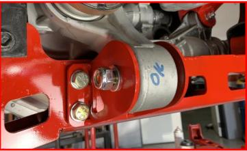
Tighten passenger differential drop bracket hardware.
