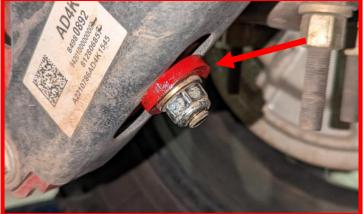
Install shock into extension using supplied M14x80mm bolt.
