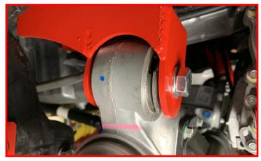
Tighten driver differential drop bracket hardware.
