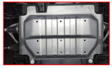
Using (2) of the factory skid plate bolts, install into the two gravel guard bolt holes.
