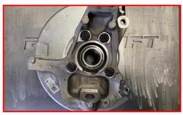
Remove the O-rings from factory knuckle, be careful not to tear the O-rings when removing.
