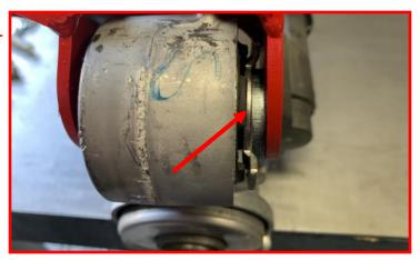
Install passenger side differential drop on factory differential mounting point using the supplied M14 x 100mm bolt, washers and nut.
