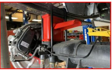
Install rear shock extensions into shock axle brackets.
