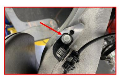
Remove brake rotor retaining bolt and remove the rotor.
