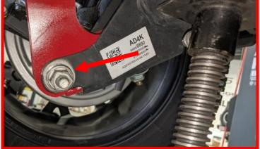
Install factory fastener between lower shock extension and lower shock axle bracket.
