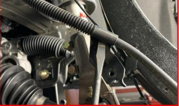
The brake line should not be strained in either direction from the brake line bracket.
