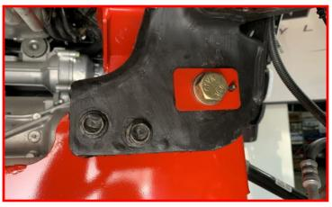
Install the (1) factory rear crossmember bolt and nut and supplied cam block off plates, M18 bolt, washers and nut through the driver side factory mount and replacement crossmember.
