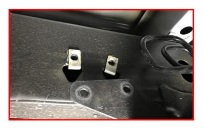
Remove ABS sensor harness bracket from top of rear differential.
