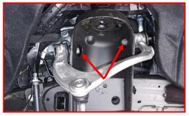
Remove (4) sway bar mounting bolts from the frame. Remove sway bar from the vehicle.
