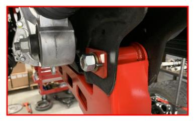
Install the heavy duty skid plate using the provided M10 bolts, washers and nuts.
