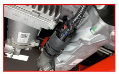
Plug in <u>electrical connector</u> on top of differential.
