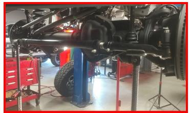
Remove the factory radius arm pivot hardware.
