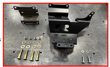
Install the center stabilizer bracket onto the differential using the supplied M8 x 30mm hex head bolts and M8 flat washers. Use the inside holes on the bracket and ensure that the bracket is flush. Tighten bolts enough to secure the bracket to the differential, but do not tighten completely at this time.
