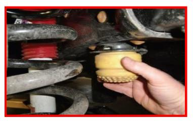
Install the ReadyLIFT bump stop spacer and factory bump stop mount to the frame using M8 x 70 mm bolt and washer.
