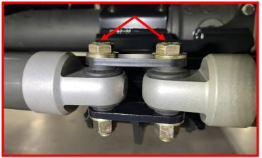
Install stabilizer shaft ends to the tie rod brackets using the M12 x 65mm bolts, washers and nuts. The shaft end will sit on top of the angled face (as shown in photo). Do not tighten at this time.
