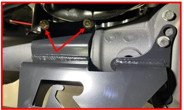
Tighten each of the four M10 nuts and bolts, making sure that the gap between each is approximately equal when tight. Tighten the M8 bolts on the differential.
