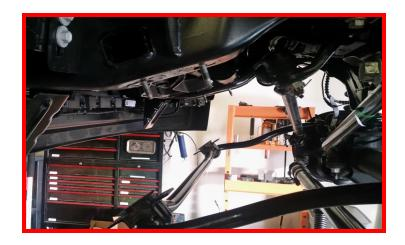
Remove track bar from the track bar bracket. Let the track bar hang out of the way. Retain factory hardware.
