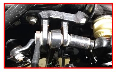
Remove the cast track bar mount on driver side of frame.
