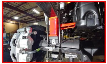
Install rear Falcon shock using factory hardware.
