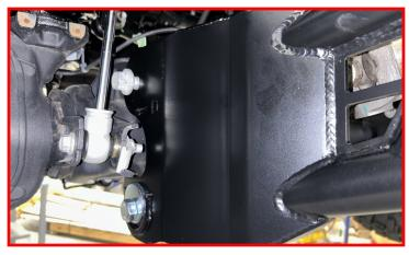
Carefully raise the radius arm into the drop bracket and secure it using the factory hardware.
