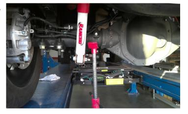
Loosen but do not remove the Ubolts one the side of the axle. This will allow slack. With a suitable jack remove the U-bolts on the opposite side and discard.
