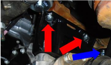
Raise the diff up to its new mounting location. Attach the passenger side bracket to the diff. Use the provided M12 bolts, washers and factory nuts.
