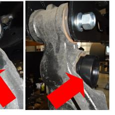
Mark the front side only of the transmission cross member where the torsion bars pass through. Mark at the 1 o'clock position and 5 o'clock position draw a 1/4" thick clearance line between these marks.
