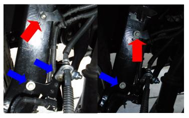
Locate the provided 12" straight end link kit. Use soapy water to add the rubber bushings and crush sleeve.
