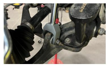
Install the outer tie rod ends to the ReadyLIFT knuckles using the factory hardware. Torque to 65 ft-lbs.
