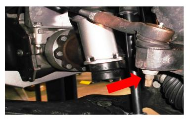
Install the extended brake line brackets. Use factory hardware to attach the bracket to the frame. Use provided hardware to attach the brake line to the bracket. Torque all brake line hardware to 20 ft-lbs.
