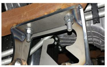
Install the ReadyLIFT driver side diff drop to the diff cradle using provided M12 bolts and washers to the forward two locations. Install the last mount using the factory bolt and a provided M12 washer and nut. Do not tighten at this time.
