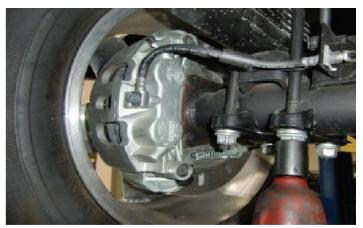
Lower the axle just enough to install the ReadyLIFT lift block. Make sure the tapered end of the block is facing forward, and the bump stop tag is inboard. Raise the axle until the block is seated in the locating pins.
