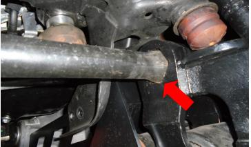
Raise the lower control arm and align the torsion bar bracket with the pervious installed torsion arm spacer. Attach the bracket to the spacer. Use provided hardware. Torque the 3/4" hardware to 250 ft-lbs.
