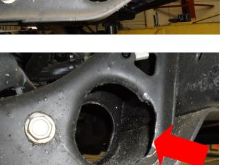
Remove the torsion bar bracket. Drill out to 7/16".
