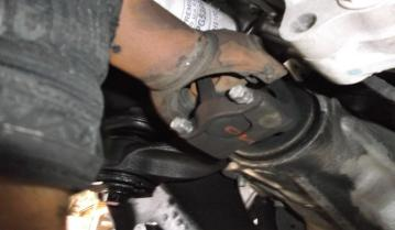
Support the differential with a suitable jack / stands, remove the driver and passenger side hardware. Mark the hardware locations as the bolts must be reinstalled in specific spots. Carefully lower the differential out of the vehicle and set aside.
