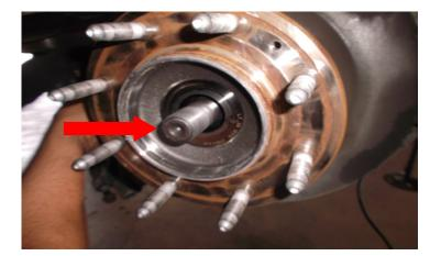
Remove the hub bearing mounting hardware from the knuckle. Make sure to not drop the hub assembly. Remove the dust shield with the assembly.
