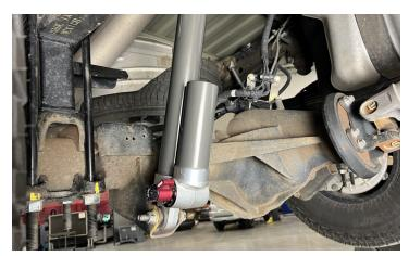
Install the provided brake line bracket to the differential. Use factory hardware. Attach the brake line to the extended bracket. Use provided hardware. Torque to 20 ft-lbs.
