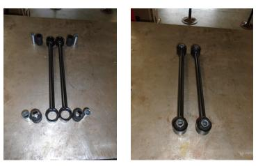
Install the assembled extended length end links. Mount the end link to the outside edge of the sway bar and the inside edge of the lower control arm. Use provided hardware. Torque to 60 ft-lbs.
