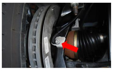
Attach the ABS wire bracket to the top hole on the knuckle. Use factory hardware. Attach the brake line and ABS wires to the provided bracket. Use supplied hardware. Attach the new bracket to the lower mount on the knuckle.
