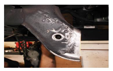
Install the ReadyLIFT passenger side diff drop to the diff cradle using the provided M12 nuts and washers. Do not tighten at this time.
