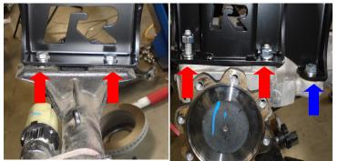
Torque all diff hardware 95 ft-lbs starting with the driver and passenger side upper hardware first. Then driver lower hardware. When tightening the passenger side lower hardware, makes sure to "center" the bracket in the diff's slotted mount. Verify that the diff clears the frame cut made earlier. If not, trim more frame material out until a minimum 1/4" clearance is gained. The frame should rest right inside the divot in the diff housing between the middle and last bolt bosses.
