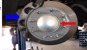
Remove the axle nut and brake rotor.
