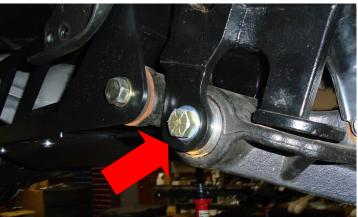
Raise the lower control arm up and support with a suitable stand. Install the ReadyLIFT knuckle to the lower and upper ball joint using the factory nuts. Torque the upper ball joint to 65 ft-lbs, and the lower ball joint to 85 ft-lbs. Transfer the o-ring from the inside of the factory knuckle to the ReadyLIFT knuckle.
