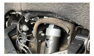
Install the lower shock mount to the lower control arm using the factory hardware.
