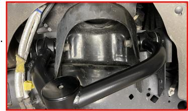
Install the coilover into the top hat using the supplied M16 Flange bolt and M16 locking flange nut.
