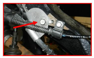
Attach the ABS bracket to the knuckle. Torque to 5 ft-lbs.
