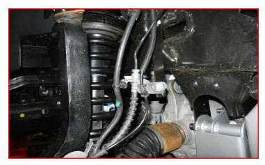
Attach the brake line to the relocation bracket using the supplied M8 x 25mm bolt, washers, and lock nut.
