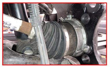
Carefully install the hub assembly over the axle shaft and into the knuckle bore. Make sure the ABS wire is located at the top of the hub.
