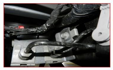
Slightly loosen but do not remove the driver side u-bolts. Remove the passenger side u-bolts completely. Lower the axle just enough to remove the factory block and install the lift block.
