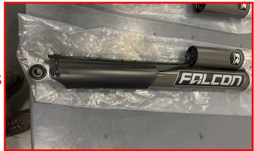
Install the roost guard using the (3) provided button head screws and thread locker.
