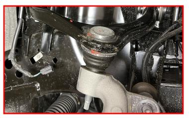
Remove the (3) bolts that attach the EIWE to the knuckle and pull both axle and the EIWE out of the factory knuckle.
