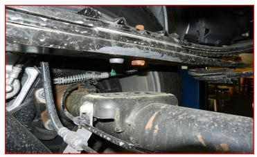
Locate the passenger side lift block, making sure the tapered end points to the front of the vehicle. Install the lift block on the axle pad aligning the pins. Raise the axle and the block up to the spring while aligning the center pins. Install the provided u-bolts, washers and nuts. Snug the u-bolt nuts but do not fully tighten at this time. Repeat steps for driver side.
