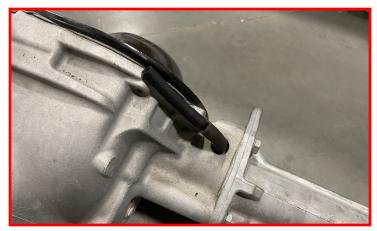
Raise differential into place. Be sure to use a helper to aid in the installation process. With the differential in place, install the factory bolt and nut through the factory driver side differential mount and the driver diff drop bracket.
