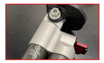
Install the completed coilover assembly into the vehicle. Be sure the lower mount is offset away from the cv axle.
