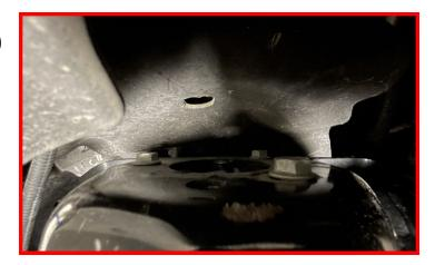
Raise the lower control arm and install the lower shock mount using the supplied hardware.
