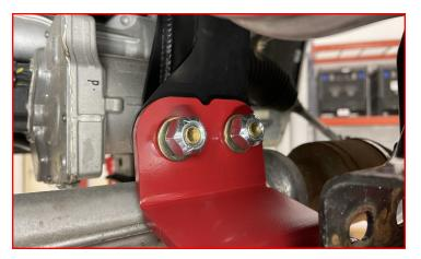
The other end of the passenger diff support bracket will install onto the rear crossmember using the provided M12 x 35mm bolt, washer and lock nut.
