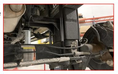
Install the rear brake line drop bracket to the frame using factory hardware. Gently pull the rear hard lines down and attach the rear brake line bracket to the drop bracket using M8 x 25mm bolt, washers, and lock nut. Torque all to 10 ft-lbs.
